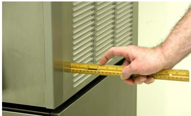
Figure 2-2 Space and Ventilation Requirements
